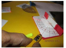
Then they pointed the toy laser beamer at the mirror along different angles on one side of the 90 degree line so that the beam glazes the surface of the paper along the folded line. Then the reflected beam on the other side of the 90 degree line was observed. Each time they found that the angle of incidence is equal to the angle of reflection. And the reflected ray grazes
