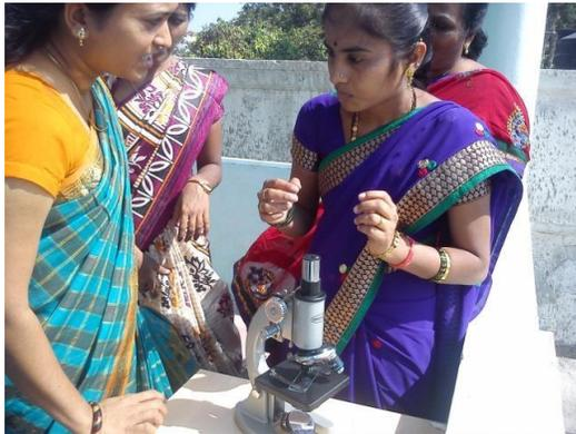
Take a thin outer layer of the onion and put it on a glass slide. Add a drop of safranin stain with ink pillar and put a coverslip on it slowly. Remove any excess stain using tissue paper and observe under the microscope.
