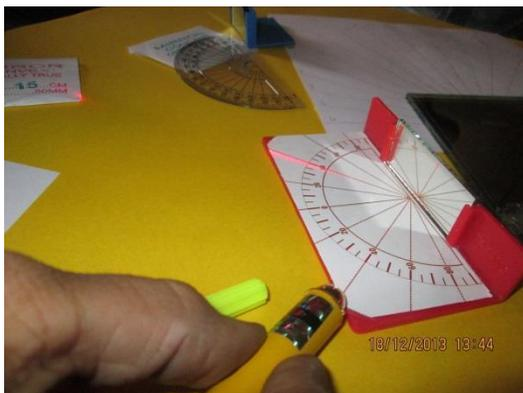
Then they pointed the toy laser beamer at the mirror along different angles on one side of the 90 degree line so that the beam grazes the surface of the paper along the folded line. Then the reflected beam on the other side of the 90 degree line was observed. Each time they found that the angle of incidence is equal to the angle of reflection. And the reflected ray grazes
